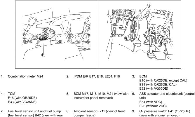
10. Oil pressure switch F41 (VQ35DE) (view with engine removed)
