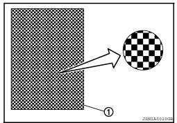
5. Push the odo/trip meter switch. Each meter/gauge should indicate as shown in the figure.
