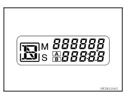
Dots in all segments of information display LCD (1) flash alternately.
