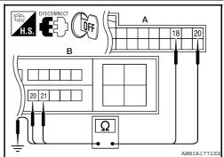
3. Check continuity between combination meter harness connector M24 (A) terminals 18, 20 and ground.
