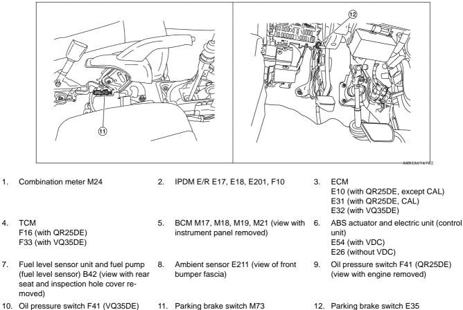
10. Oil pressure switch F41 (VQ35DE) (view with engine removed)
