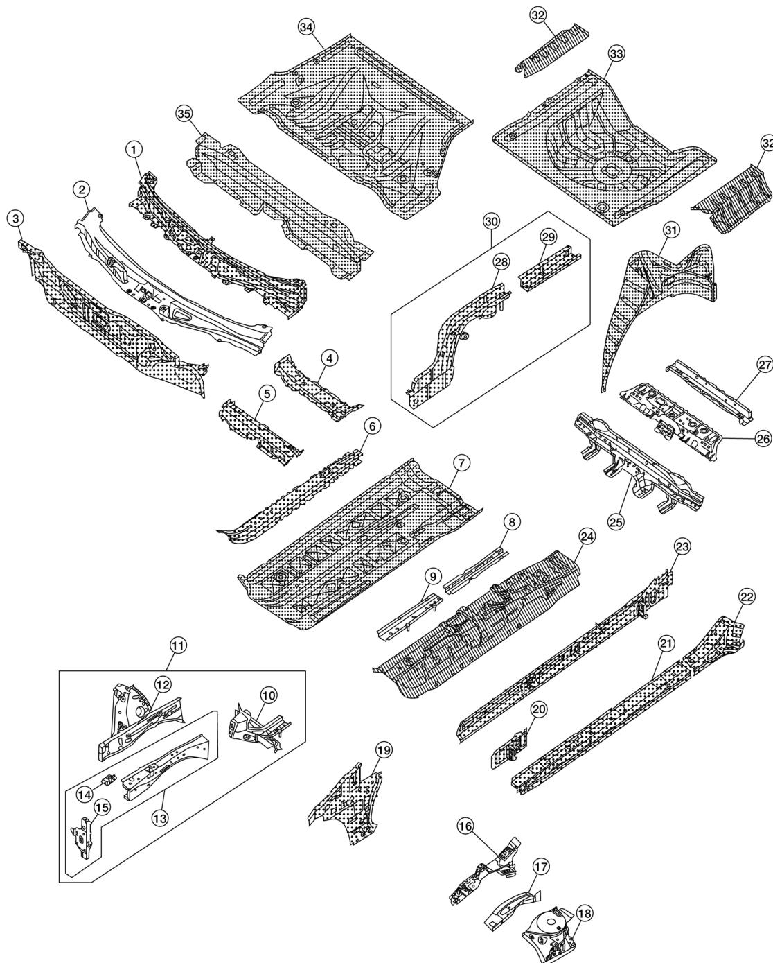
■ : Indicates both-sided anti-corrosive precoated steel portions
