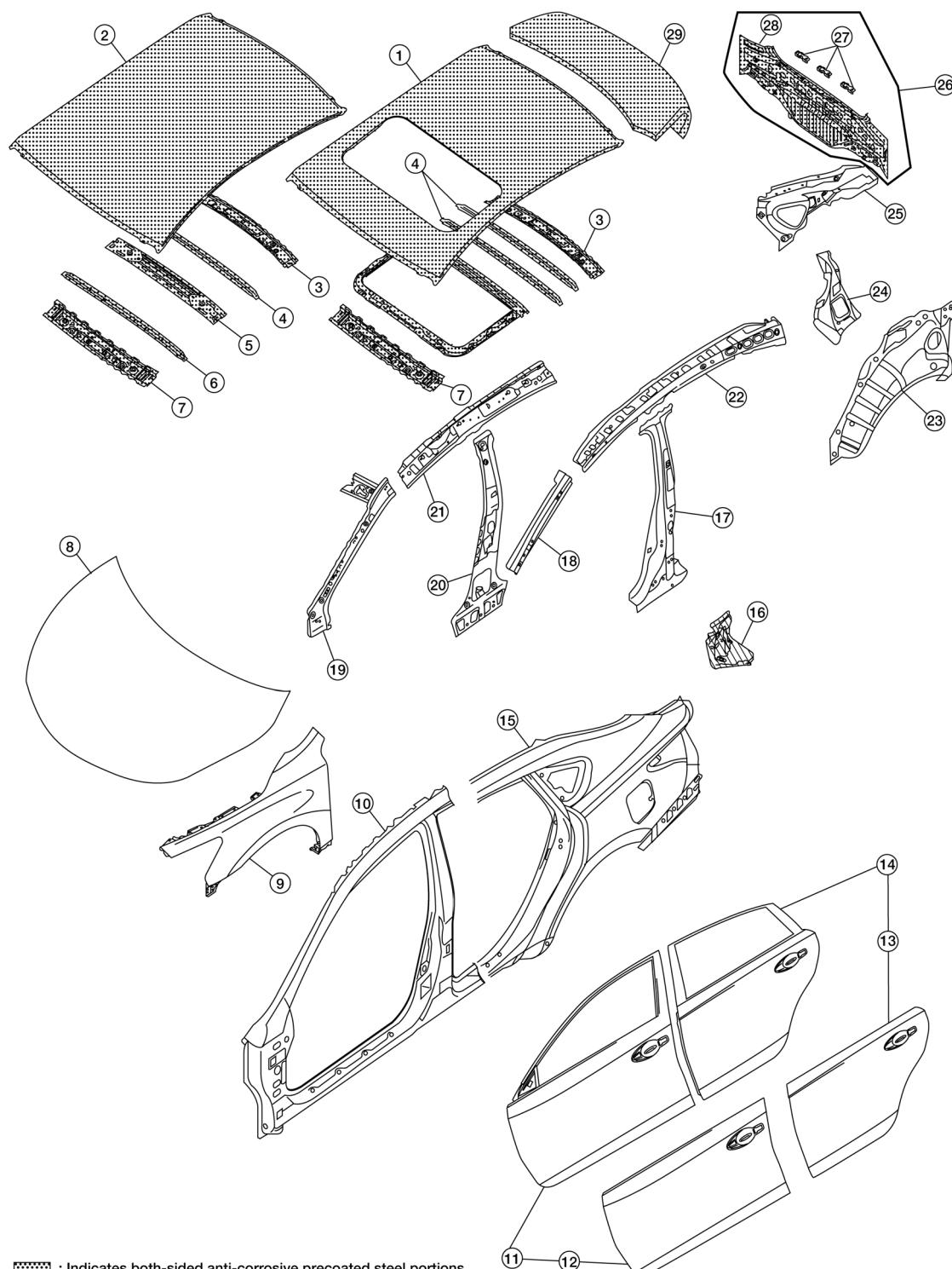
■ : Indicates both-sided anti-corrosive precoated steel portions
