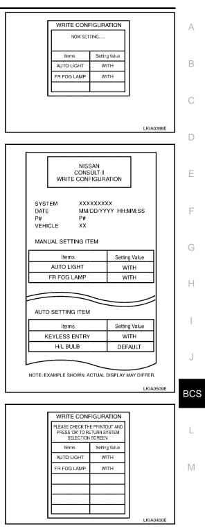
WRITE CONFIGURATION results are printed out automatically. Confirm "WRITE CONFIGURATION" is correctly executed by comparing sheet automatically printed out with applicable configuration list shown in step 9.
