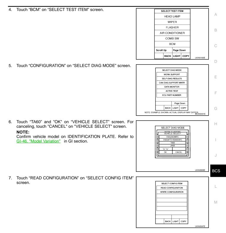
Configuration of current BCM is printed out automatically. A listing of manual setting items and auto setting items will be displayed. Auto setting items are preset and cannot be changed. Manual setting items can be set by using WRITE CONFIGURA-TION PROCEDURE. Refer to <u>BCS-16, "WRITE CONFIGURA-TION PROCEDURE"</u>.
