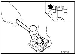
4. Remove the bearing at the opposite side in above operation.
