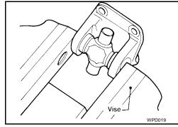
2. Select snap rings that will provide the specified play in an axial direction of the journal, and install them. Refer to <a href="PR-13">PR-13</a>, "Snap Ring"</a>.
