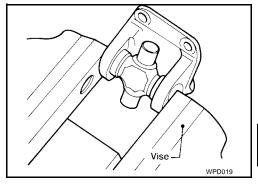
2. Select snap rings that will provide the specified play in an axial direction of the journal, and install them. Refer to <a href="PR-13">PR-13</a>, "Snap Ring" .
