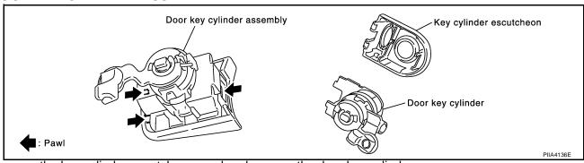
Remove the key cylinder escutcheon pawl and remove the door key cylinder.
