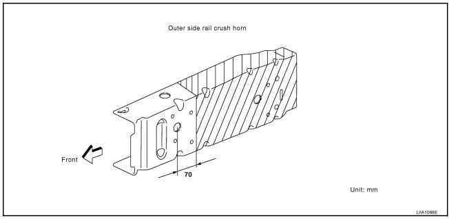
Scribe a straight line on the outer side rail crush horn along the hole center as shown in the figure. Cut off outer side rail crush horn along scribed line.
