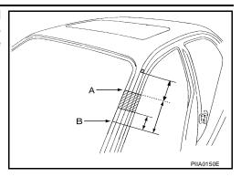
Determine cutting position and record distance from the locating indent. Use this distance when cutting the service part. Cut outer front pillar over 60 mm above inner front pillar cut position.
