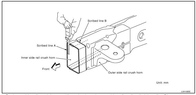
• Cut inner side rail crush horn at 45 mm backward cut position of cut line A. (along line B)
