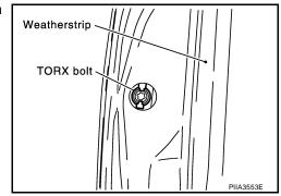
4. While pulling the outside handle, remove the door key cylinder assembly or escutcheon.
