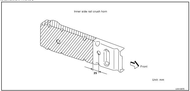
Scribe a straight line on the inner side rail crush horn along the hole center as shown in the figure. Cut off inner side rail crush horn along scribed line.
