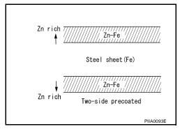
Nissan Genuine Service Parts are fabricated from galvannealed steel. Therefore, it is recommended that GENUINE NISSAN PARTS or equivalent be used for panel replacement to maintain the anti-corrosive performance built into the vehicle at the factory.
