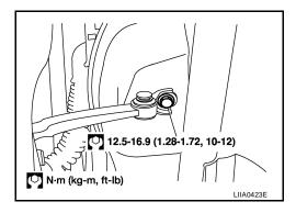
5. Remove the door-side hinge nuts and bolts, and remove the door assembly.
