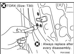
9. While pulling the outside handle bracket, slide it toward the rear of vehicle to remove it and the door lock assembly.
