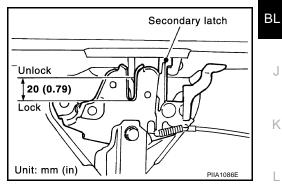
Check the hood lock lubrication condition. If necessary, apply "body grease" to the points shown in the figure.
