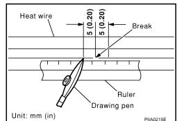
4. After repair has been completed, check repaired wire for continuity. This check should be conducted 10 minutes after silver composition is deposited.
