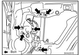
2. Install the glass from outside to ensure that it is in both the front and rear glass channels. Tighten glass bolts to the specified torque.
