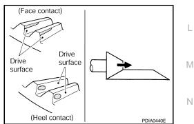
• If the tooth contact is near the flank (flank contact), or near the toe (toe contact), use a thinner drive pinion height adjusting washer to move the drive pinion farther from the drive gear. Refer to DLN-225, "Inspection and Adjustment".
