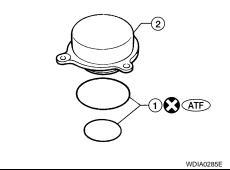
4. Install the oil filter to the transfer assembly. Tighten the bolts to the specified torque. Refer to DLN-125, "Removal and Installation".
