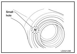
8. Remove the front oil seal using Tool as shown.
