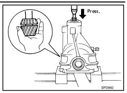
8. Remove the drive pinion rear bearing inner race and drive pinion height adjusting washer using Tool.
