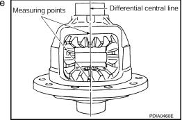
Using feeler gauges, measure the clearance between the side gear back and differential case at three different points, while rotating the side gear. Average the three readings to calculate the clearance. (Measure the clearance of the other side as well.)
