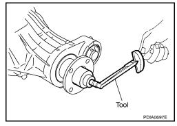
• If the measured value is out of the specification, check and adjust each part. Adjust the drive pinion bearing preload torque first, then adjust the side bearing preload torque.
