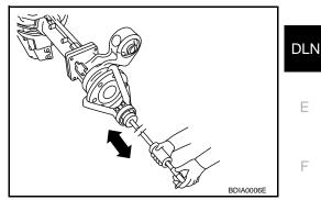
3. Place a small hole in the side oil seal case using suitable tool.
