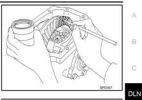
2. Rotate the drive gear back and forth several times. Then check for correct drive pinion to drive gear tooth contact as shown. CAUTION:
