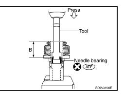
3. Apply ATF to the circumference of the new metal bushing and install it to the sun gear assembly using Tool.
