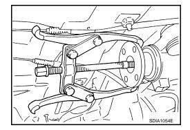
8. Remove the front oil seal using Tool.
