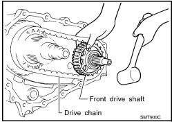
4. Remove the front drive shaft front bearing using Tools.
