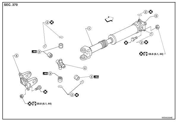
Propeller shaft tube 1.
