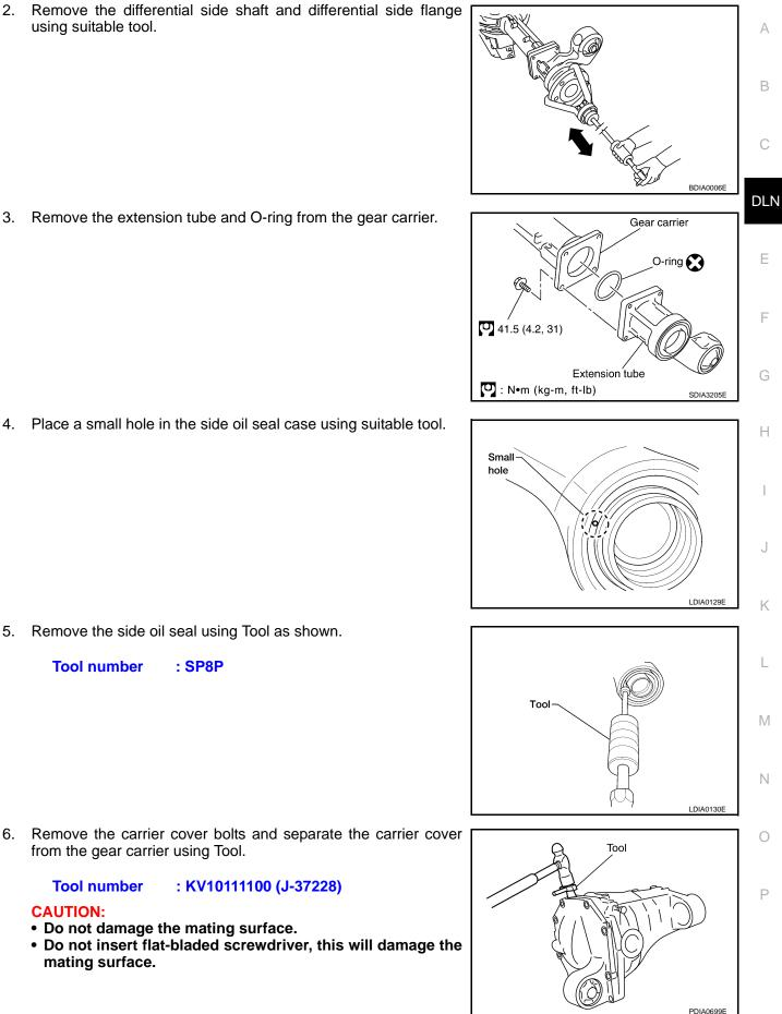
Remove the extension tube and O-ring from the gear carrier. 3.
