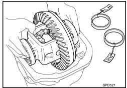
11. Remove side bearing inner race using Tools as shown.
