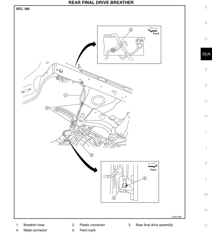
• Fill the rear final drive assembly with differential gear oil after installation. Refer to DLN-235.
