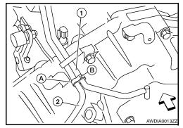
7. Install the transfer air breather hose into the breather tube (transfer, metal connector) until the hose end reaches the base of the tube. Set transfer air breather hose with paint mark facing upwards.
