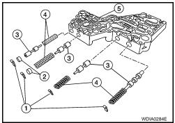
Install each control valve (3), springs (4), and plugs (2) to the C. upper body (5), and install retainer plates (1) to hold them in place.
