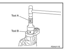
2. Install drive pinion front bearing outer race using Tools.
