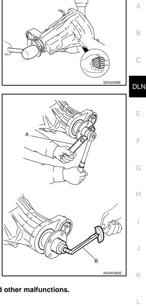
Apply anti-corrosive oil to the threads of the drive pinion and the seating surface of the new drive pinion lock nut. Then adjust the drive pinion lock nut tightening torque using Tool (A), and check the drive pinion bearing preload torque using Tool (B).
