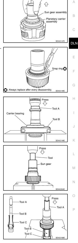
28. Remove the snap ring from the sun gear assembly using suitable tool.
