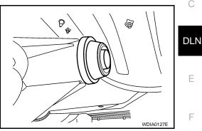
Remove the rear oil seal from the rear case using Tool. 4.
