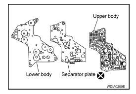
Install the lower body and separator plate to the upper body. e. CAUTION: Do not reuse separator plates.
