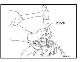
16. Remove the pinion mate shaft.
