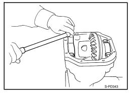
7. Lift the differential case assembly out using Tool.
