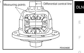
2. Using feeler gauges, measure the clearance between the side gear back and differential case at three different points, while rotating the side gear. Average the three readings to calculate the clearance. (Measure the clearance of the other side as well.)
