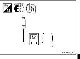
3. Check continuity between the license plate lamp harness connectors and ground.
