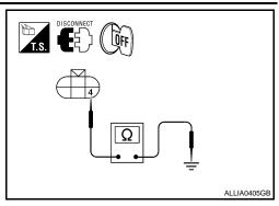
2. Check continuity between the rear combination lamp harnness connectors and ground.
