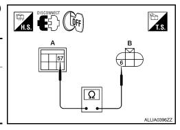
4. Check continuity between the IPDM E/R harness connector (A) and the rear combination lamp harness connector (B).
