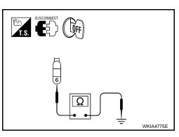
3. Check continuity between the door mirrors and ground (if equipped with turn signals in the mirrors).
