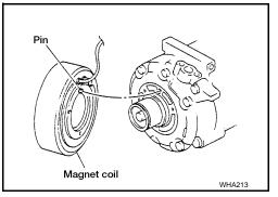
2. Install the magnet coil harness clip using a screwdriver.
