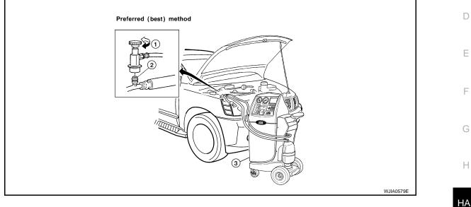
Shut-off valve 1. 2. A/C service valve 3. Recovery/recycling equipment
