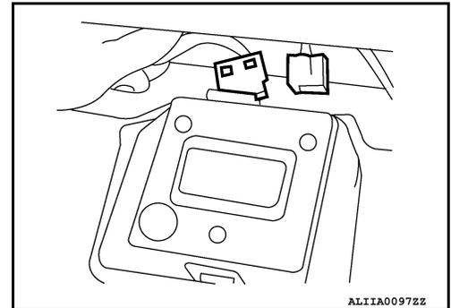
5. Press the front release tab and remove the seat control unit.
