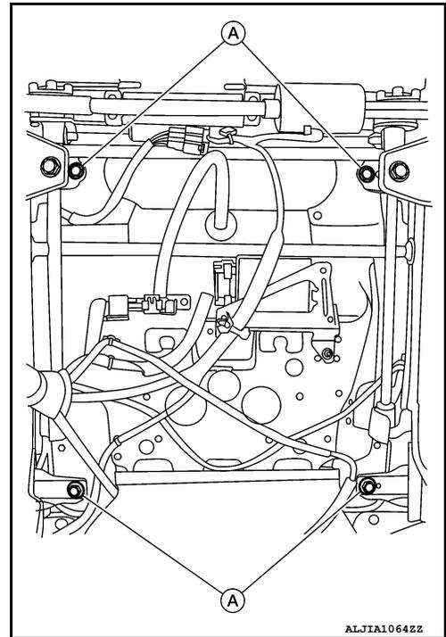
4. Remove the seat cushion trim and seat cushion pad as an assembly from the seat cushion frame.
