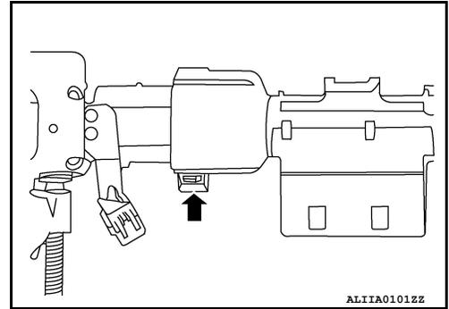
8. Remove the power seat cross beam screws and the power seat cross beam.
