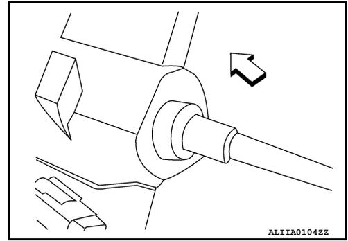
2. Install the power seat cable (A) into the seat motor.
