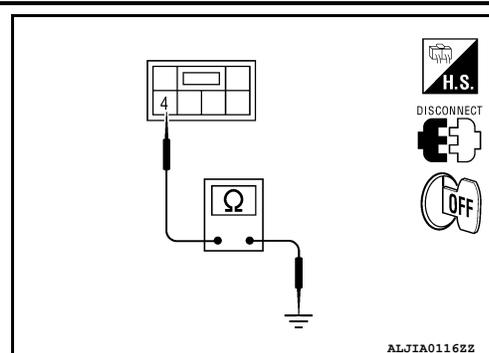
4. Check continuity between any third row power folding seat switch passenger side harness connector B162 or B163 terminals 2, 3 and third row power folding seat control unit harness connector B401 terminals 3, 11.
