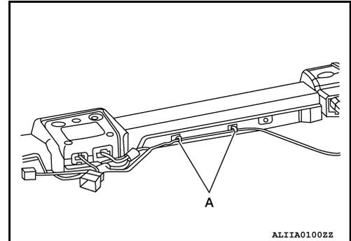
8. Install the seat control unit and connect the seat control unit harness connectors.
