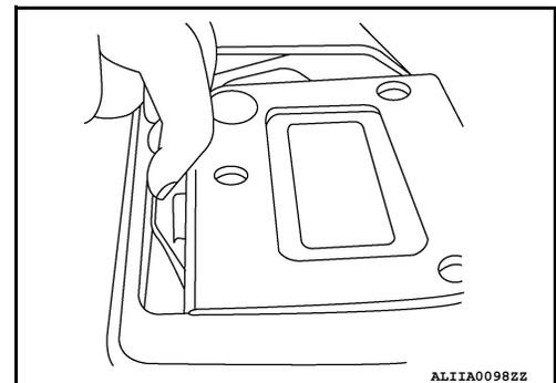
5. Unclip the wiring harness from the seat motor cover clips (A).
