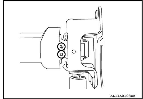
9. Remove the power seat cable from the power seat cross beam.
