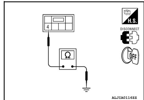
4. Check continuity between any third row power folding seat switch driver side harness connector B164 or B165 terminals 2, 3 and third row power folding seat control unit harness connector B401 terminals 4, 12.
