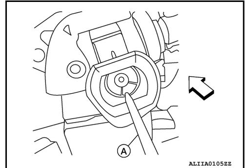
3. Install the power seat cross beam RH side screws
