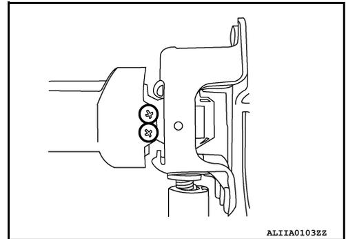
4. Starting at the RH side, snap the power seat cable into the power seat cross beam retainer clips.
