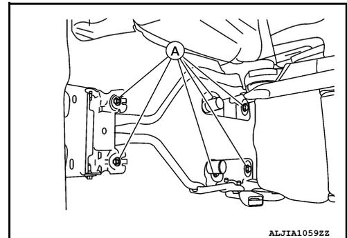
3. Tilt the seat cushion back in the locked position and remove the seat.
