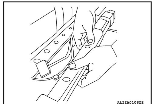
5. Snap the hinged strap retainer around the seat motor.
