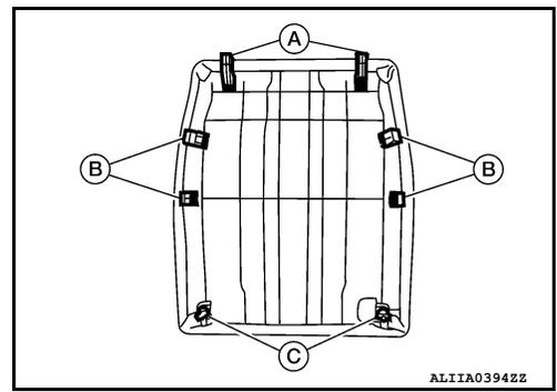
3. Hold the seatback board as shown and pull the top of the seatback board away from the seatback frame.
