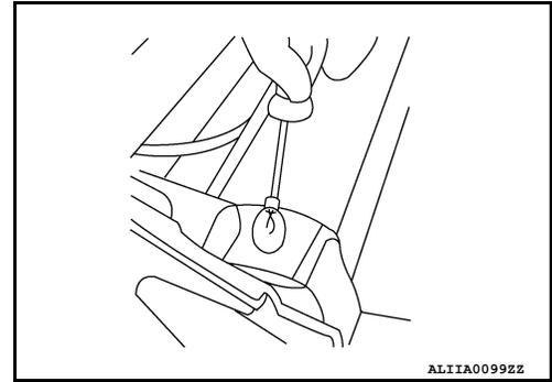
7. Install the seat harness to the seat motor cover clips (A).
