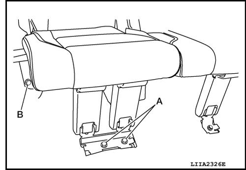
4. Remove the seat cushion side facing retainer clip and release elastic band from seat belt buckle.
