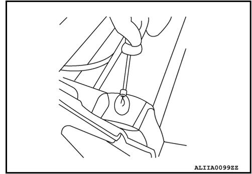
7. Release the power seat cross beam clip and open the hinged strap.
