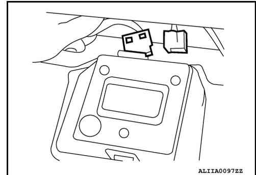
4. Press the front release tab and remove the seat control unit.
