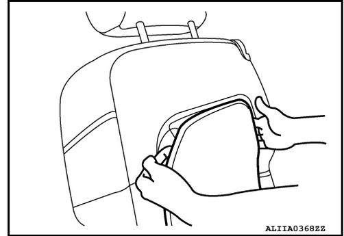
4. Pull the middle part of the seatback board to disengage the side tabs from the seatback frame.
