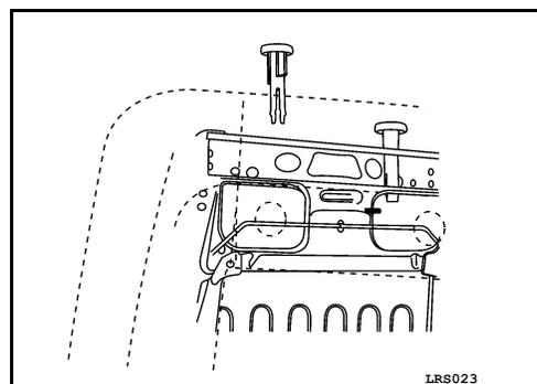
4. Remove the snap ring and the lumbar support lever knob (if equipped).
