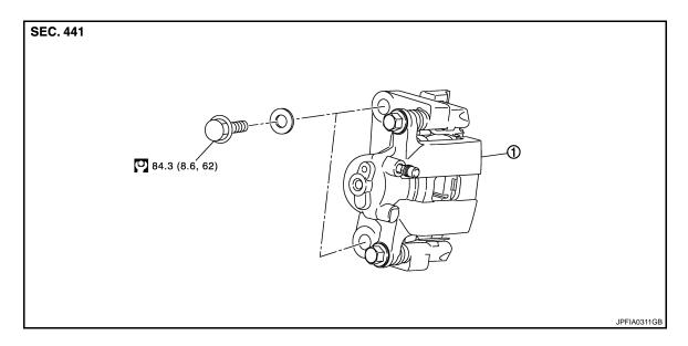
1. Brake caliper assembly
