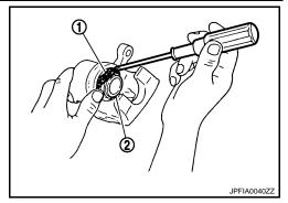
4. Apply brake fluid to piston (1). Push piston into cylinder body by hand and push piston boot (2) piston side lip into the piston groove.
