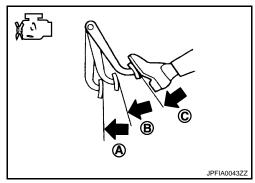
Depress the brake pedal with the engine running. Then stop the engine while holding down the brake pedal. Check that the brake pedal stroke does not change after holding down the brake pedal for 30 seconds or more.
