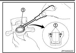
7. Place a wooden block as shown in the figure, and blow air from union bolt mounting hole to remove piston and piston boot. **CAUTION:**
