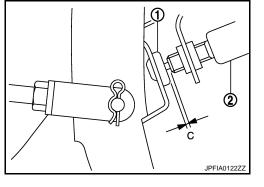
Depressed Brake Pedal Height Check the brake pedal height (H2) between the dash lower panel (1) and the brake pedal upper surface when depressing the brake pedal at 490 N (50 kg, 110 lb) while turning engine ON.
