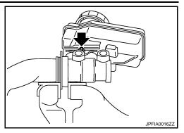
4. Tilt the reservoir tank so that a mounting pin can be inserted. Insert a mounting pin. Return the reservoir tank to the horizontal position. Insert another mounting pin into the pin hole on the opposite side in the same manner after the mounting pin passes through the cylinder body pin hole.
