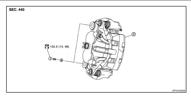
Brake caliper assembly
