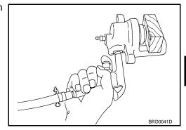
Remove piston seal from cylinder body using suitable tool. CAUTION:
