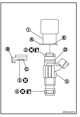
5. Install fuel tube and fuel injector assembly to intake manifold. **CAUTION:**
