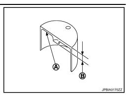
Available thickness of valve lifter: 27 sizes with range 7.88 to 8.40 mm (0.3102 to 0.3307 in) in steps of 0.02 mm (0.0008 in) (when manufactured at factory). Refer to <u>EM-140, "Camshaft"</u>.
