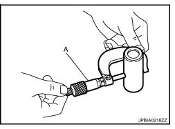
Piston to Piston Pin Oil Clearance (Piston to piston pin oil clearance) = (Piston pin hole diameter) – (Piston pin outer diameter)
