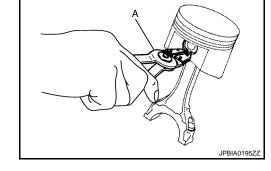
b. Heat piston to 60 to 70°C (140 to 158°F) with an industrial use drier (A) or equivalent.
