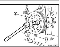
Place suitable puller tab on holes of crankshaft pulley, and pull e. crankshaft pulley through. **CAUTION:**
