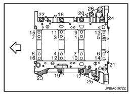
e. Turn lower cylinder block bolt (No. 1 to 16) 90 degrees clockwise (angle tightening). CAUTION:
