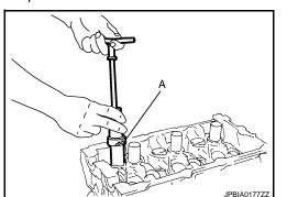
9. Remove valve seat, if valve seat must be replaced.
