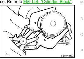
7. Remove piston from connecting rod as follows:
