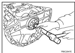
• Press-fit pilot converter with its chamfer facing crankshaft as shown in the figure.
