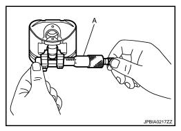
Piston Pin Outer Diameter Measure the outer diameter of piston pin with a micrometer (A).
