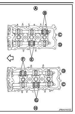
d. Rotate crankshaft 240 degrees clockwise (when viewed from engine front) to align No. 5 cylinder at TDC of compression stroke.
