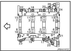
9. Remove lower cylinder block as follows:
