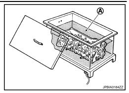
c. Provide valve seats cooled well with dry ice. Force fit valve seat into cylinder head. **WARNING:**
