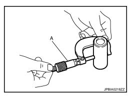
Connecting Rod Bushing Oil Clearance
