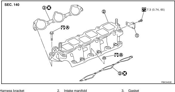
1. Harness bracket 2. Intake manifold
