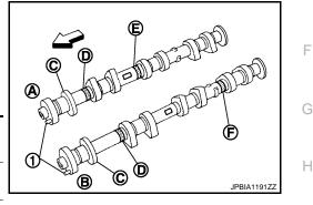
• Install camshaft so that dowel pin (A) on front end face are positioned as shown in the figure. (No. 1 cylinder TDC on its compression stroke)
