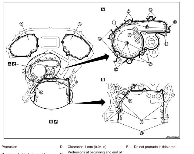
F. Run along bolt hole inner side
