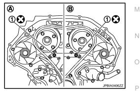
9. Install new front oil seal on front timing chain case.
