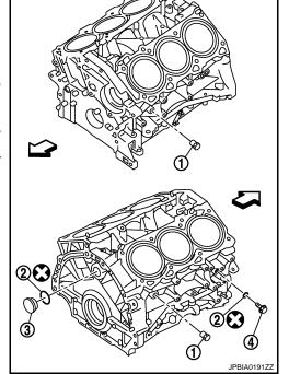
• Tighten each plug as specified below.
