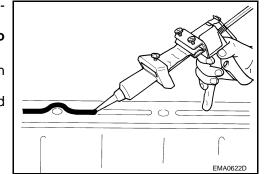
3. Attach liquid gasket tube to the tube presser (commercial service tool).
