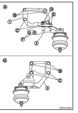
Tighten rear engine mounting member bolts in numerical order as shown in the figure.
