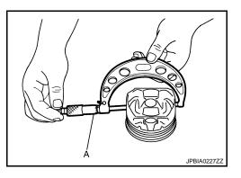
Piston-to-Cylinder Bore Clearance
