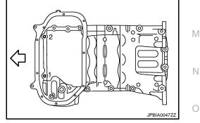
29. Remove front timing chain case as follows:
