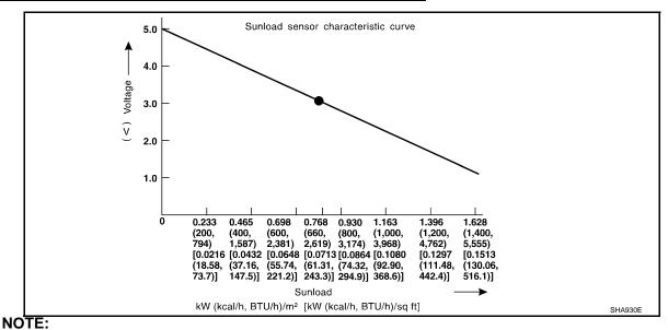
Select a place where sunshine directly on it when checking sunload sensor.
