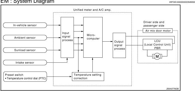
WITH LEFT AND RIGHT VENTILATION TEMPERATURE SEPARATELY CONTROL
