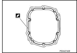
24. Install carrier cover on gear carrier and tighten mounting bolts.
