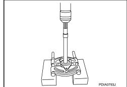
2. Remove side shaft oil seal (1) from extension tube retainer with a suitable tool.
