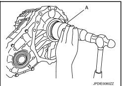
23. Install front oil seal until it is flush with end face of front case with the drift (A) [SST: ST27862000 ( — )].
