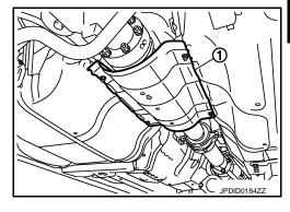
5. Put matching marks ( onto propeller shaft rubber coupling and final drive companion flange.
