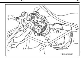
Remove front oil seal using the puller (A) [SST: KV381054S0 (J-34286)].
