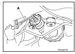
9. Put matching mark (B) on the end of the drive pinion. The matching mark should be in line with the matching mark (A) on companion flange (1).
