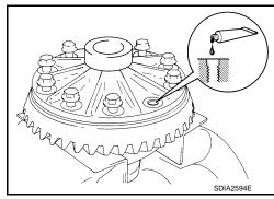
9. Install drive gear on the mounting bolts.
