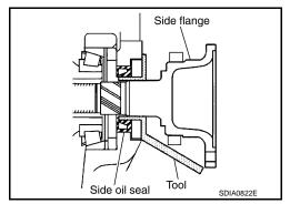
Put a suitable drift on the center of side flange, then drive it until sound changes.
