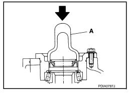
20. Using the drift (A) [SST: KV38102100 (J-25803-01)], press-fit side oil seal so that its surface comes face-to-face with the end surface of gear carrier.
