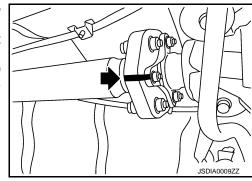
If propeller shaft or final drive has been replaced, connect them as follows:
