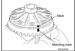
9. Apply thread locking sealant into the thread hole of drive gear.
