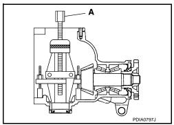
13. Remove side bearing inner race.
