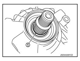
19. Install rear oil seal to rear case with the drifts within the dimension (L) shown as follows.
