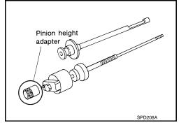
8. Position the side bearing discs, J-25269-4, and arbor firmly into the side bearing bores. Install the bearing caps and tighten bearing cap mounting bolts to the specified torque. Refer to <u>DLN-198</u>, "AWD: Exploded View".
