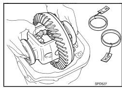
14. Insert selected left and right side bearing adjusting washers in place between side bearings and gear carrier. Refer to <u>DLN-171</u>, "2WD: Adjustment".
