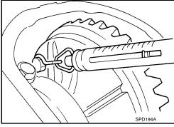
If the turning torque is outside the specification, use a thicker/ thinner side bearing adjusting washer to adjust.
