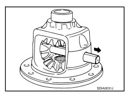
19. Turn pinion mate gear, then remove pinion mate gears, pinion mate thrust washers, side gears and side gear thrust washers from differential case.
