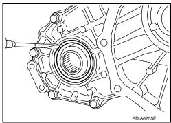
5. Put a matching mark (A) on the end of mainshaft. The mark should be in line with the mark (B) on the companion flange. **CAUTION:**
