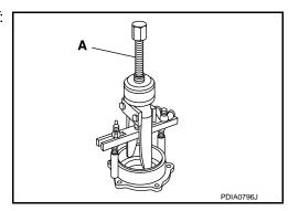
12. Remove side bearing outer race with puller (A) [SST: KV381054S0 (J-34286)].
