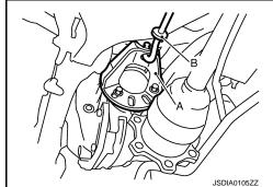
8. Measure the total preload with the preload gauge (A) [SST: ST3127S000 (J-25765-A)].
