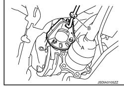
Remove side oil seal, using a suitable tool. CAUTION:
