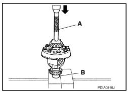
Press-fit side bearing outer race into side retainer with the drift and the drift bar.
