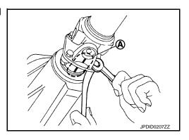
Align matching marks (A) to install propeller shaft rebro joint and final drive companion flange.
