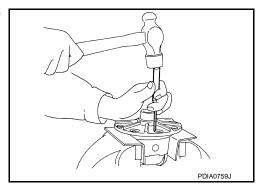
14. Remove pinion mate shaft.
