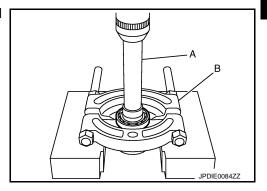
Remove front drive shaft rear bearing with the drift (A) and puller (B).
