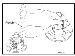
Align the matching mark of differential case with the mark of drive gear, then place drive gear.
