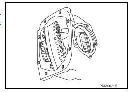
15. Install selected side bearing adjusting shim (1). Refer to <u>DLN-120, "Adjustment"</u>.
