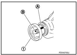
10. Apply anti-corrosion oil to the thread and seat of drive pinion lock nut, and temporarily tighten drive pinion lock nut to drive pinion.
