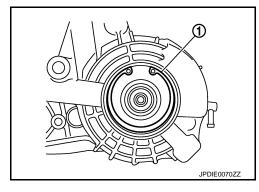
21. Remove rear bearing from rear case with the drifts.
