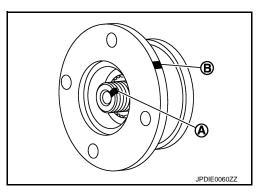
6. Remove companion flange with a puller (A) (commercial service tool).
