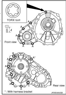
10. Remove front case (1) from rear case by levering it up with a suitable tool.
