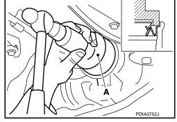
3. Align the matching mark (B) of drive pinion with the matching mark (A) of companion flange (1), and then install the companion flange.
