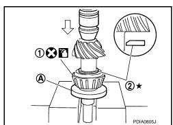
4. Assemble collapsible spacer to drive pinion. **CAUTION**:
