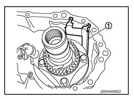
15. Remove oil cover bolts from rear case. And then, remove oil cover (1).
