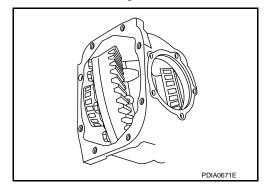
4. Install side bearing adjusting shim before disassembling or shim which thickness is the same as the one before disassembling.
