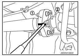
9. Remove center bearing mounting bracket fixing nuts.
