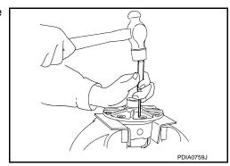
14. Remove pinion mate shaft.
