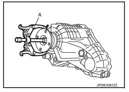
7. Remove rear oil seal from rear case with the puller (A) [SST: KV381054S0 (J-34286)].
