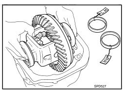
14. Insert selected left and right side bearing adjusting washers in place between side bearings and gear carrier. Refer to <u>DLN-184</u>, "AWD: Adjustment".
