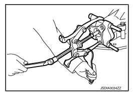
Press drive pinion assembly out of gear carrier. CAUTION:
