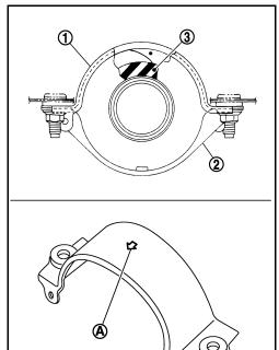
Align matching marks (A) to install propeller shaft flange yoke and transfer companion flange.
