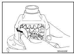
4. Align the lock pin holes on differential case with shaft, and install pinion mate shaft.
