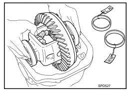
9. Remove side bearing inner race.
