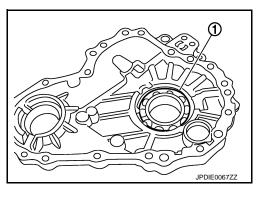
15. Apply liquid gasket to mating surface of rear case.
