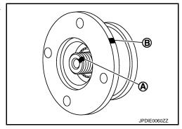
4. Remove the companion flange with a puller (A) (commercial service tool).
