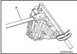
22. Install mainshaft oil seal until it is flush with end face of front case with the drift (A) [SST: ST30720000 (J-25405)].
