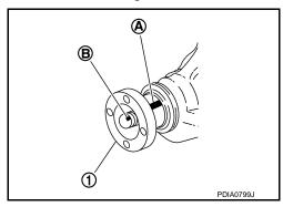
Temporarily tighten removed drive pinion lock nut to drive pinion.
