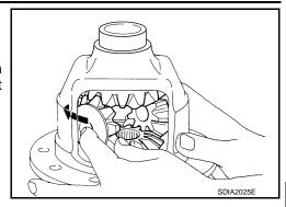
5. Align the lock pin holes on differential case with shaft, and install pinion mate shaft.
