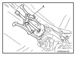
5. Remove the rear oil seal with the puller (A) [SST: KV381054S0 (J-34286)].
