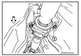
7. Remove propeller shaft assembly fixing bolts and nuts ( ). CAUTION:
