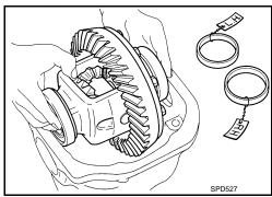
9. Remove side bearing inner race.
