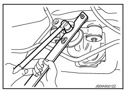
11. Remove companion flange using pullers.
