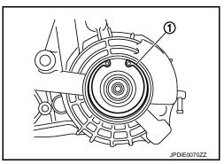
5. Install mainshaft assembly to rear case with the drift (A) [SST: ST35321000 ( — )].
