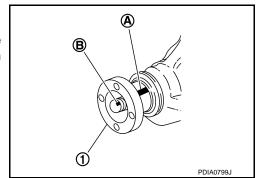
Apply anti-corrosion oil to the thread and seat of new drive pinion lock nut, and temporarily tighten drive pinion lock nut to drive pinion.
