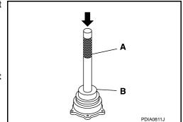
12. Press-fit side bearing outer race into gear carrier with the drift and the drift bar.
