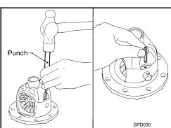
Align the matching mark of drive gear with the mark of differential case, then place drive gear.
