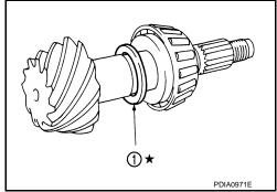
3. Install selected pinion height adjusting washer (2) to drive pinion. Press pinion rear bearing inner race (1) to it, using drift (A) [SST: ST30032000 (J-26010-01)].
