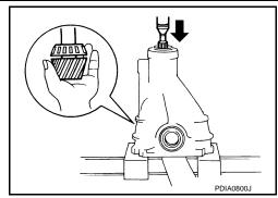
Remove pinion rear bearing inner race and pinion height adjusting washer with replacer (A) (commercial service tool).
