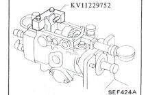
(6) Push tension lever until it comes into contact with stopper pin. Back governor sleeve up until start lever contacts tension lever. At this point, read dial gauge.
