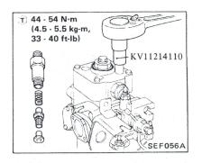
(11) Install spring seat, spring and E-ring.
