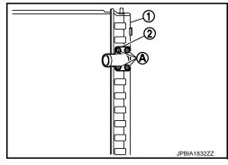
6. Rotate two radiator upper mount brackets 90 degrees in direction as shown in the figure, and remove them.
