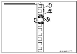
6. Rotate two radiator upper mount brackets 90 degrees in direction as shown in the figure, and remove them.
