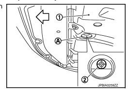
When draining all of engine coolant in the system, open water drain plugs on cylinder block. Refer to EM-92, "Setting".
