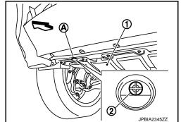
When draining all of engine coolant in the system, open water drain plug on cylinder block. Refer to <a href="EM-202">EM-202</a>, "Setting".
