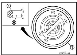
Install thermostat with jiggle valve (A) facing upwards. The position deviation may be within the range of 20 degrees (b).
