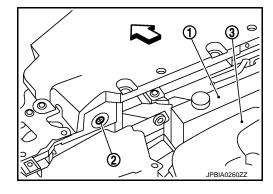
5. Remove air relief plug (1) on heater hose.
