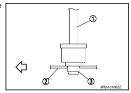
b. Remove radiator (1) from front of radiator core support (2).
