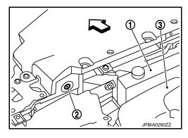
Remove air relief plug (1) on heater hose. (models with air relief plug on heater hose)
