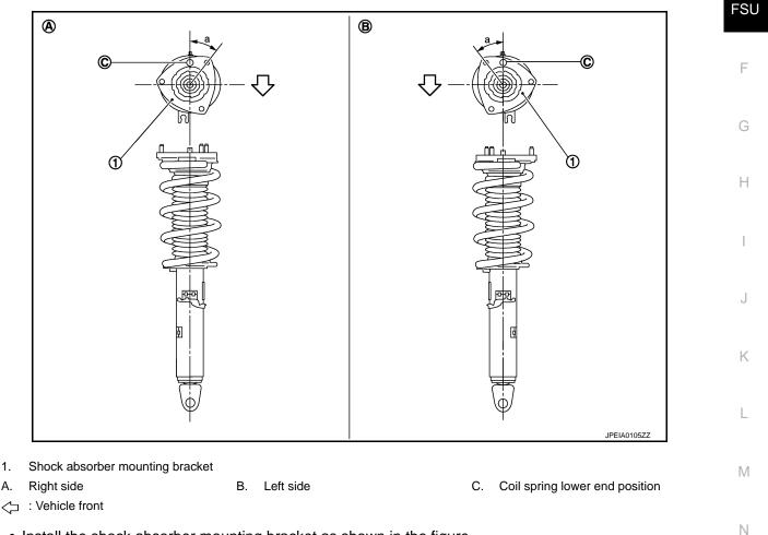
• Install the shock absorber mounting bracket as shown in the figure.
