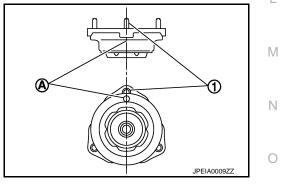
6. Insert bound bumper into shock absorber mounting bracket, and then install it to shock absorber together with rubber seat.
