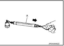
Rotating Torque Inspection
