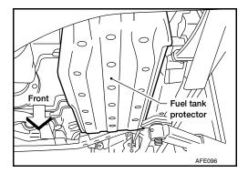
9. Remove fuel tank mounting bolts while supporting fuel tank.
