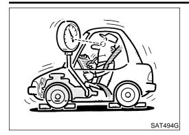
Start engine and measure line pressure at idle and stall speed.
