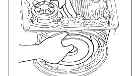
16. Remove front side clutch and gear components.
