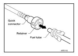
Insert tube into the center of the connector until you hear a click.
