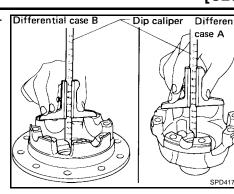
Measure thickness of each disc and plate. Number of discs and plates (One side), Friction disc 5, Friction plate 6 and Spring plate 2.
