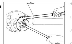
10. Tighten the pinion nut by very small degrees until the specified preload is achieved. When checking the preload, turn the drive pinion in both directions several times to set the bearing rollers.
