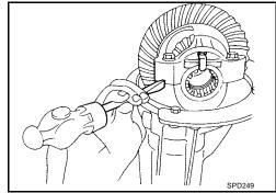
2. Put match marks on one side of side bearing cap with paint or punch to ensure that it is replaced in proper position during reassembly.
