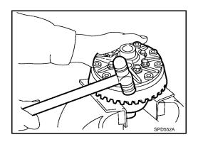
Press Tool • Put matching marks on component parts so that they can be reinstalled in their original positions from which they were Matching mark
