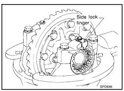
7. Check runout of ring gear with a dial indicator.
