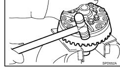
4. Remove couple bolts on differential cases A and B with a press.
