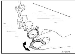
4. Measure frictional surfaces and projected portions of friction disc, friction plate, spring plate, and determine each part's differences to see if the specified wear limit has been exceeded.
