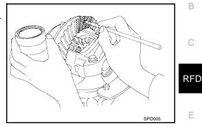
3. Hold companion flange steady by hand and rotate the ring gear in both directions.
