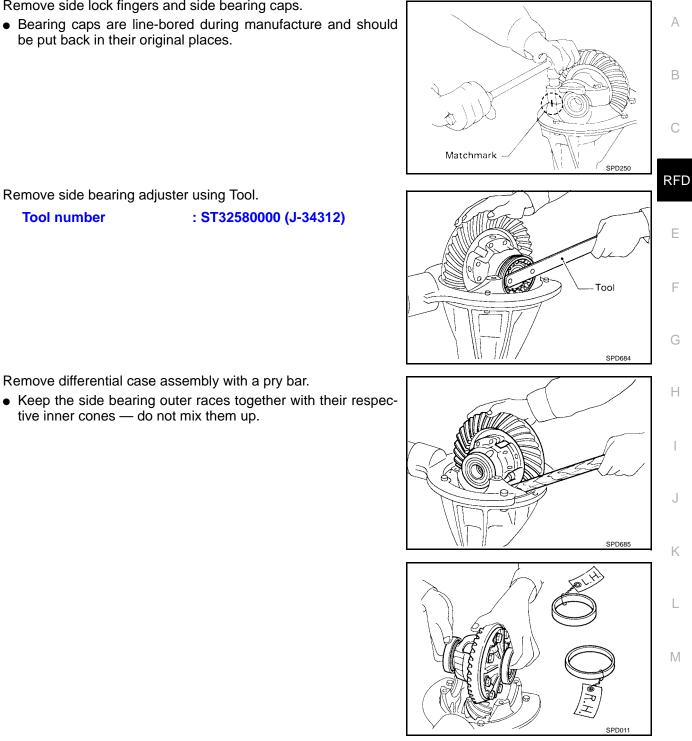
4. Remove side bearing adjuster using Tool. : ST32580000 (J-34312) **Tool number**
