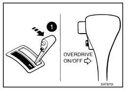
7. Release the overdrive control switch (the O/D OFF indicator lamp will begin to flash ON and OFF).
