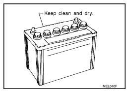
When the vehicle is not going to be used over a long period of time, disconnect the negative battery terminal. (If the vehicle has an extended storage switch, turn it off.)
