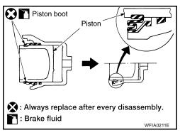
3. Insert into cylinder body by hand and insert piston boot piston-side lip into piston groove.
