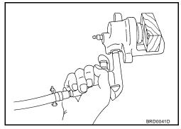
Using a flat-bladed screwdriver, remove piston seal from cylinder body.
