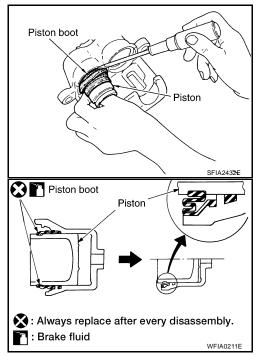
4. Insert into cylinder body by hand and insert piston boot piston-side lip into piston groove.
