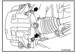
Install brake hose to brake caliper assembly, if removed, then tighten union bolt to the specified torque. Refer to <u>BR-22</u>, "Components".
