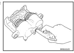
Using a flat-bladed screwdriver, remove piston seal from cylinder body.
