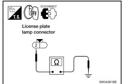
5. Check continuity between rear combination lamp (tail) harness connector and ground.
