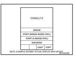
3. Touch "BCM" on "SELECT SYSTEM" screen. If "BCM" is not indicated, go to <u>GI-40, "CONSULT-II Data Link</u> <u>Connector (DLC) Circuit"</u>.
