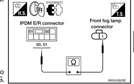
NG >> Check for short circuits and open circuits in harness between IPDM E/R and front fog lamps.
