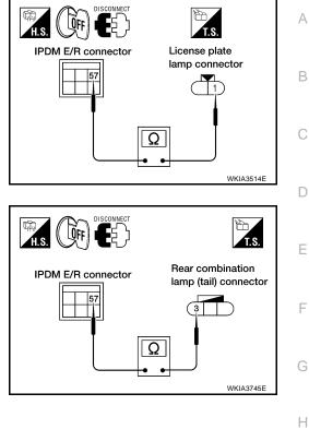
6. Check continuity between IPDM E/R harness connector and rear combination lamp (tail) harness connector.
