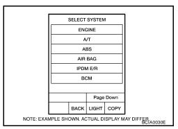
4. Select the desired part to be diagnosed on the "SELECT DIAG MODE" screen.
