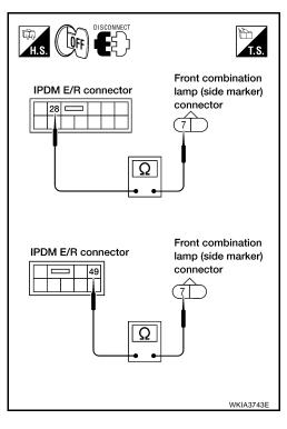
4. Check continuity between IPDM E/R harness connector and front combination lamp (parking) harness connector.
