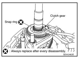
21. Install the snap ring to the mainshaft, using suitable tool.
