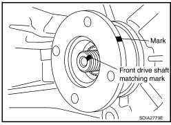
5. Remove the companion flange, using suitable tool.
