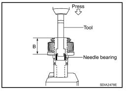
3. Install the carrier bearing to the sun gear, using Tools.
