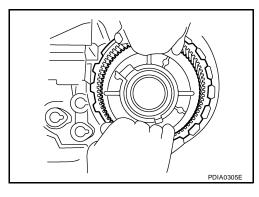
35. Remove the snap ring from the front case.
