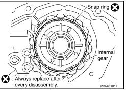
7. Install the planetary carrier assembly and sun gear assembly to the front case, using Tool.
