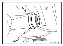
4. Remove the rear oil seal from the rear case, using Tool.
