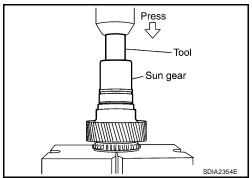
6. Remove the metal bushing from the sun gear, using Tools.
