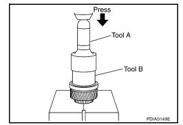
4. Install the snap ring to the sun gear assembly, using suitable tool.
