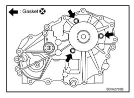
15. Remove the rear case bolts and harness bracket from the rear case.
