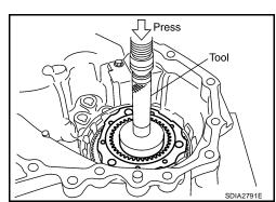
8. Install the snap ring to the sun gear.
