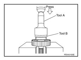
2. Install the front bearing, using Tools.
