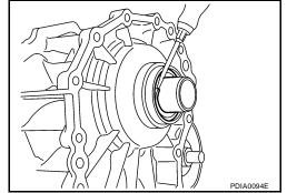
14. Remove the retainer bolts and gaskets.
