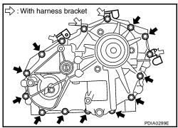
29. Install the retainer bolts with new gaskets. Tighten the bolts to the specified torque. Refer to TF-110, "COMPONENTS".
