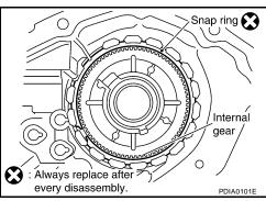
34. Remove the internal gear from the front case.
