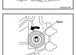
b. Align the transfer control device shaft cutout with the mark on the control shift rod, and install it.
