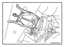
6. Remove the front oil seal from the front case, using Tool.
