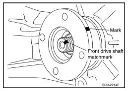
3. Install the self-lock nut and tighten to the specified torque, using Tool. Refer to  $\overline{\text{TF-110}}$ , "COMPONENTS".
