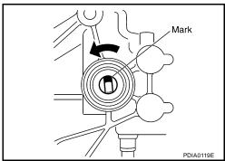
b. Align the transfer control device shaft cutout with the mark on the control shift rod, and install.
