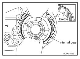
6. Install the snap ring to the front case.
