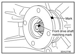
6. Remove the companion flange, using suitable tool.
