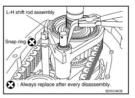
19. Install the snap ring to the mainshaft, using suitable tool.
