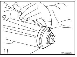
12. Remove the rear oil seal from the rear case, using Tool.
