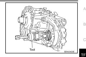
8. Remove the 4LO switch [gray (with green paint)] and ATP switch (black) from the front case.
