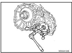
Remove the front oil seal from the front case, using Tool.
