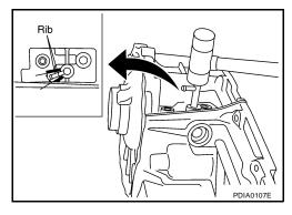
2. Install the baffle plate to the front case. Tighten the bolt to the specified torque. Refer to <a href="https://example.com/TF-110">TF-110</a>, "COMPONENTS"</a>.
