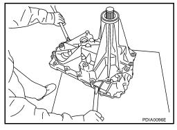
18. Remove the snap ring from the mainshaft, using suitable tool.
