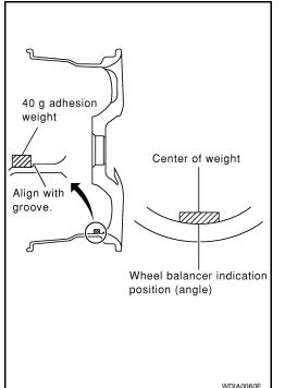
c. If calculated balance weight value exceeds 50 g (1.76 oz), install two balance weight sheets in line with each other as shown.
