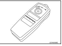
7. Register the IDs in order from FR LH, FR RH, RR RH and RR LH. When ID registration of each wheel has been completed, a buzzer sounds and the warning lamp flashes.
