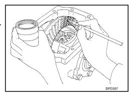
3. Rotate drive gear back and forth several times, check drive pinion gear to drive gear tooth contact.
