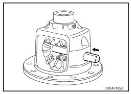
6. Drive a lock pin into pinion mate shaft, using punch. Make sure lock pin is flush with differential case.
