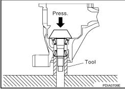
8. Using the drift, install front oil seal until it becomes flush with the case end.
