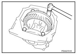
6. Lift differential case assembly out with suitable tool.
