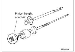
Position the side bearing discs, J-25269-18, and arbor firmly into the side bearing bores. Install the bearing caps and tighten bearing cap bolts to the specified torque. Refer to <a href="FFD-16">FFD-16</a>, "COMPO-NENTS"
