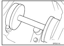
Select the correct standard pinion height adjusting washer thickness. Select by using a standard gauge of 3 mm (0.12 in) and your J-34309-101 feeler gauge. Measure the distance between the J-34309-10 pinion height adapter including the standard gauge and the arbor.
