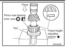
4. Assemble collapsible spacer to drive pinion.
