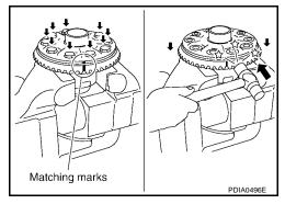
12. Remove lock pin of pinion mate shaft with punch from drive gear
