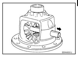
14. Turn pinion mate gear, then remove pinion mate gear, pinion mate thrust washer, side gear and side gear thrust washer from differential case.
