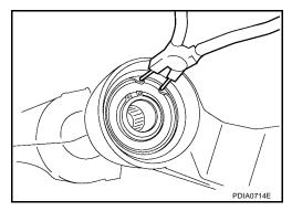
4. Remove side shaft assembly out of gear carrier.
