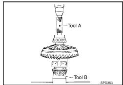
11. Install housing spacer.
