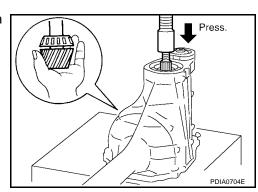
7. Remove pinion rear bearing inner race and drive pinion height adjusting washer.
