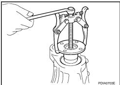
6. Press drive pinion assembly out of gear carrier. (Together with collapsible spacer.)
