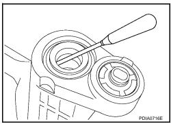
11. Tap pinion front/rear bearing outer races uniformly a brass rod or equivalent to removed.
