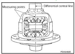
2. Using feeler gauge, measure the clearance between side gear back and differential case at 3 different points, while rotating side gear. Average the 3 readings, and then measure the clearance. (Measure the clearance of the other side as well.)
