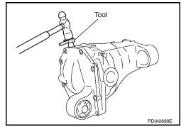
I. For proper reinstallation, paint matching marks on one side of the bearing cap.
