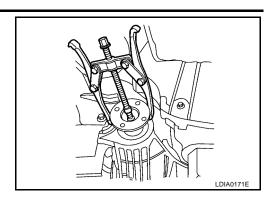
13. Remove the front oil seal using Tool.
