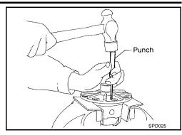
13. Remove pinion mate shaft.
