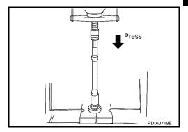
5. Using the drift, drive side oil seals until it becomes flush with the case end.
