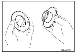
2. Install side gears and thrust washers into differential case.
