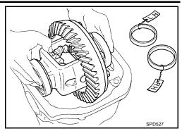
13. Insert left and right original side bearing adjusting washers in place between side bearings and gear carrier, with tool.
