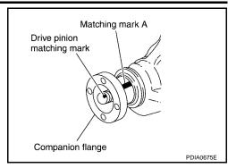
10. Apply gear oil to the thread and seat of drive pinion lock nut, and temporarily tighten drive pinion lock nut to drive pinion.
