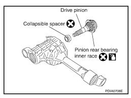
6. Apply gear oil to pinion front bearing, and assemble pinion front bearing inner race to drive pinion assembly.
