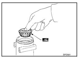
7. Using the drift, press the pinion front bearing inner race to drive pinion as far as drive pinion lock nut can be tightened.
