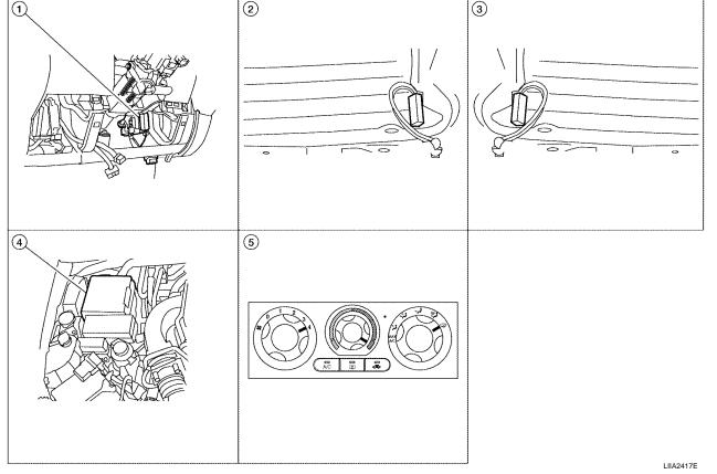
BCM M18, M20 (view with instrument lower panel LH removed)
