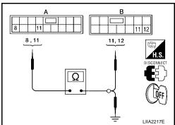
3. Check continuity between main power window and door lock/unlock switch connector and ground.
