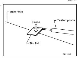
2. Attach probe circuit tester (in Volt range) to middle portion of each filament.
