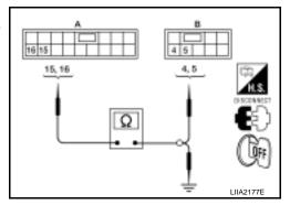
Check continuity between main power window and door lock/ unlock switch and ground.
