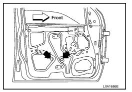
7. While holding the door window, raise it at the rear and pull the glass out of the sash toward the outside of the door.
