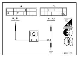
4. Check continuity between main power window and door lock/unlock switch connector and ground.
