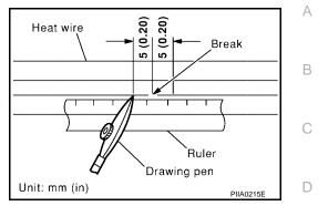
After repair has been completed, check repaired wire for continuity. This check should be conducted 10 minutes after silver composition is deposited.
