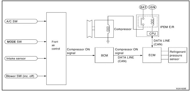
When the A/C switch is pressed, or the mode switch is turned to the defroster position, the front air control outputs a compressor ON signal to BCM.
