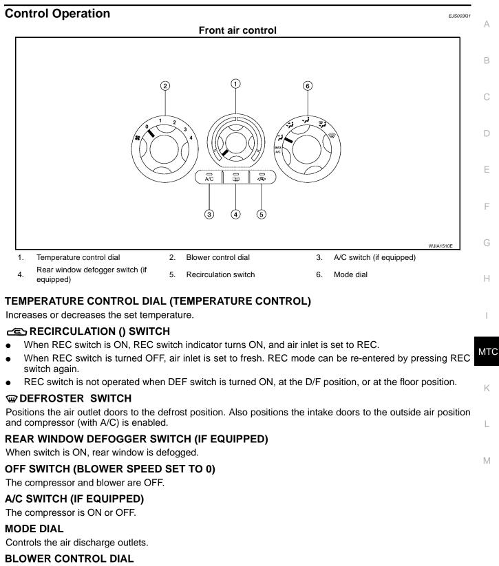
Manually controls the four blower speeds, and turns blower off and on.
