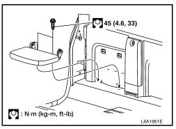
3. Remove the bolt, lift and remove the seatback assembly.
