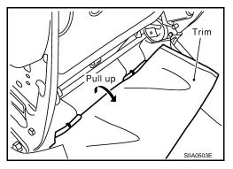
6. Remove the retainer on the seat cushion frame, then remove the harness connector for the seat cushion heater (if equipped).
