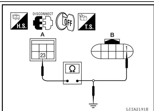
4. Check continuity between IPDM E/R harness connector E120 (A) terminal 23 and ground.
