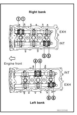
5. For the measured value out of the standard, perform adjustment.
