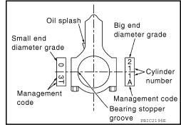
2. Apply crankshaft pin journal diameter grade stamped on crankshaft front side to the column in the "Connecting Rod Bearing (No. 1 - 5 from left) Pin journal diameter grade (No. 1 - 4 from left)
