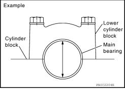
If the clearance exceeds the limit, select proper main bearing according to main bearing inner diameter and crankshaft main journal diameter to obtain the specified bearing oil clearance. Refer to <u>EM-101</u>, "How to <u>Select Piston and Bearing</u>".
