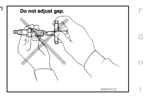
INSTALLATION Installation is in the reverse order of removal. CAUTION: Do not drop or shock the spark plug.
