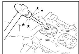
3. Ream cylinder head valve guide hole using suitable tool.
