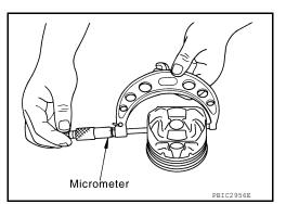
Piston to Cylinder Bore Clearance
