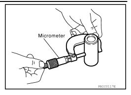
Connecting Rod Bushing Oil Clearance
