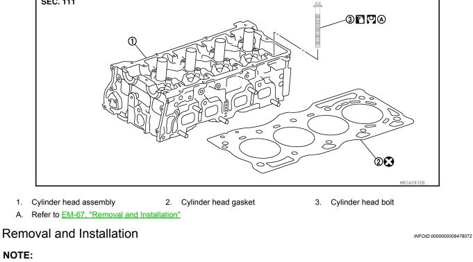
When removing components such as hoses, tubes/lines, etc., cap or plug openings to prevent fluid from spilling.
