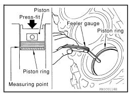
• If the measured value exceeds the limit, replace piston ring, and measure again.
