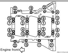
ii. Turn M10 bolts 90° clockwise in numerical order from No. 1 to 16 using Tool.
