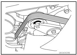
INSTALLATION Installation is in the reverse order of removal. CAUTION: Make sure belt is securely installed around all pulleys.
