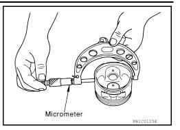
Piston to Cylinder Bore Clearance
