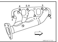
5. Remove exhaust manifold (RH) and exhaust manifold cover (RH) together.
