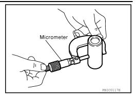
Piston to Piston Pin Oil Clearance
