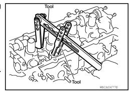
Valve spring (with valve spring seat)
