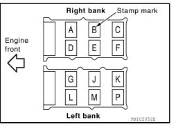
Apply liquid gasket to mating surface of camshaft bracket (No. 1) as shown on right and left banks. Use Genuine RTV Silicone Sealant or equivalent. Refer to GI-21, "Recommended Chemical Products and Sealants".
