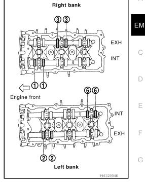
Rotate crankshaft by 240° clockwise (when viewed from engine C. front) to align No. 3 cylinder at TDC of its compression stroke. NOTE:
