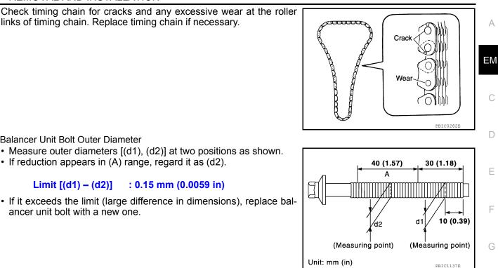
Balancer Unit Bolt Outer Diameter
