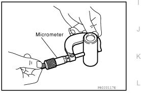
Piston to Piston Pin Oil Clearance (Piston to piston pin oil clearance) = (Piston pin hole diameter) – (Piston pin outer diameter)
