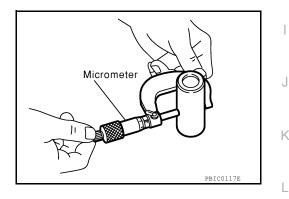
Connecting Rod Bushing Oil Clearance (Small End)
