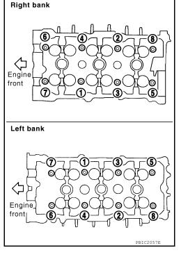
Measure the tightening angle using Tool.
