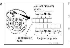
When Crankshaft and Connecting Rod are Reused
