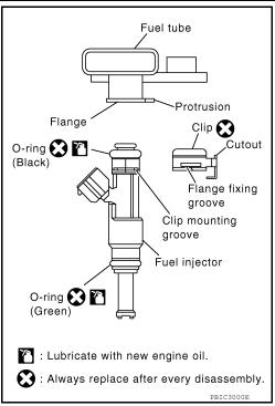
3. Install fuel tube and fuel injector assembly as follows: CAUTION:
