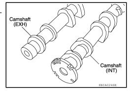
• Install camshafts so that camshaft dowel pins on the front side are positioned as shown.
