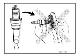
• If the spark plug tip is covered with carbon, spark plug cleaner may be used.
