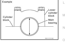
If the calculated value exceeds the limit, select proper main bearing according to main bearing inner diameter and crankshaft main journal diameter to obtain specified bearing oil clearance. Refer to EM-242, "How to Select Piston and Bearing".
