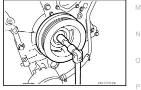
c. Pull crankshaft pulley with both hands to remove it.
