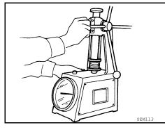
• If the installation load or load with valve open is out of the standard, replace valve spring.
