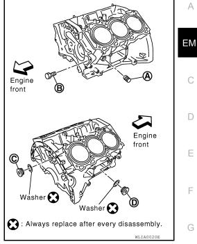
Tighten each plug as specified below.
