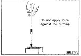
While holding the wire of the male terminal, try to insert the male terminal into the female terminal. Do not force the male terminal into the female terminal with your hands.
