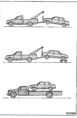
INFINITI recommends that the vehicle be towed with the driving (front) wheels off the ground as illustrated.
