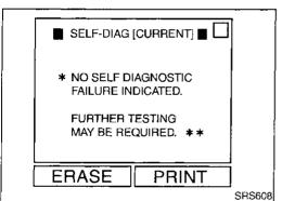
7. If no malfunction is detected on "SELF-DIAG [CURRENT]", repair of SRS is completed.
