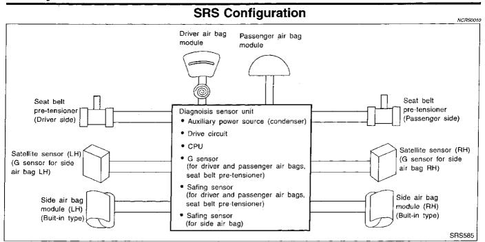
The air bag deploys if the diagnosis sensor unit activates while the ignition switch is in the "ON" or "START" position.
