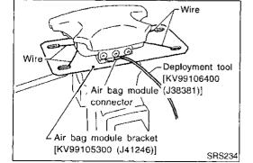
3. Connect deployment tool [SST: KV99106400 (J38381)] to air bag module connector.
