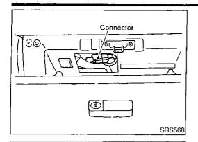
Connect air bag module connector to air bag harness connector.
