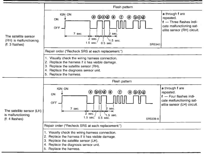
\* Follow the procedures in numerical order when repairing malfunctioning parts. Confirm whether malfunction is eliminated using the air bag warning lamp or CONSULT each time repair is finished. If malfunction is still observed, proceed to the next step. When malfunction is eliminated, further repair work is not required.
