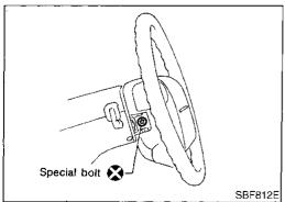
Remove side lids. Using the TAMPER RESISTANT TORX (Size T50), remove left and right special bolts. Air bag module can then be removed.
