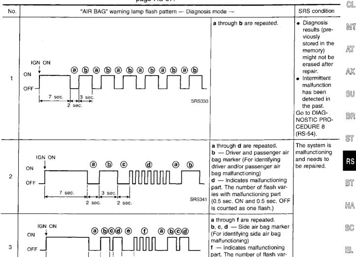
Malfunctioning part is indicated by the number of flashes (part d or f). Compare the number of flashes to "Air Bag Warning Lamp Flash Code Chart", page RS-50, and locate malfunctioning part.
