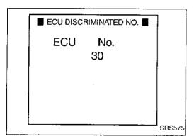
For INFINITI G20, the diagnosis sensor unit classification number assigned is 30.
