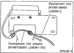
Connect deployment tool adapter [SST: KV99108300 (J38381-35)] to deployment tool [SST: KV99106400 (J38381)] connector and connector on air bag module.
