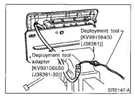
Connect red clip of deployment tool to battery positive termi-
