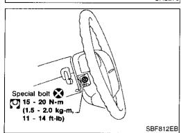
Unlock the spiral cable connector. Then disconnect connectors and remove the four screws. The spiral cable can then be removed.
