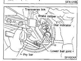
e) Hold flanges of third link with both hands. Twist third link fully to the right and read dial gauge indication. Similarly, twist third link to the left and read dial gauge indication.
