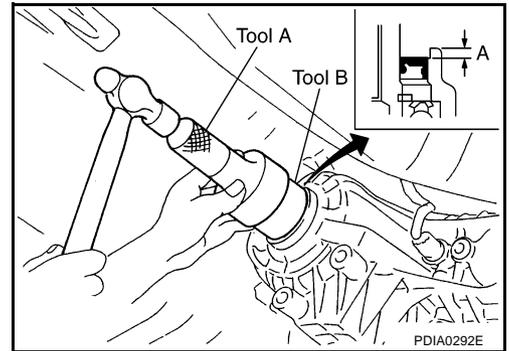
2. Align the matchmark of mainshaft with the mark of companion flange, then install the companion flange.
