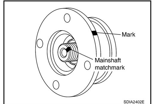
3. Using flange wrench, install the self-lock nut of companion flange and tighten to the specified torque. Refer to [TF-50, "COMPONENTS"](#).
