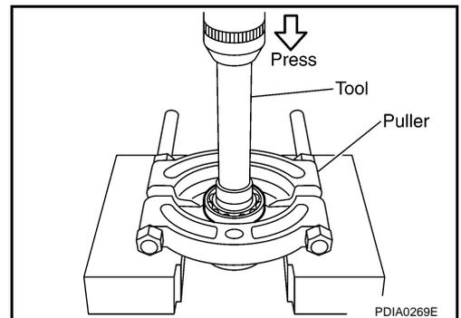
4. Remove front drive shaft rear bearing, using drift and puller.
