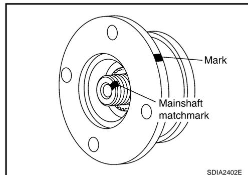
22. Tighten self-lock nut to the specified torque, with flange wrench. Refer to [TF-50, "COMPONENTS"](#).
