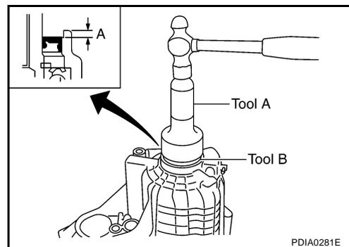
21. Install companion flange while align the matchmark of mainshaft with the mark of companion flange.
