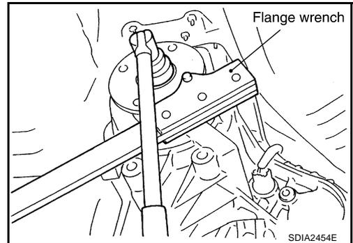
3. Put matchmark on the end of the mainshaft. The mark should be in line with the mark on the companion flange.
