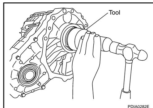
24. Install front oil seal until it is flush with end face of front case, using drift.
