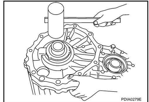
18. Tighten front case and rear case fixing bolts to the specified torque. Refer to [TF-50, "COMPONENTS"](#).
