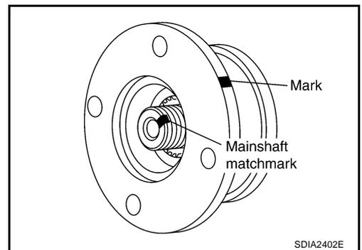
6. Remove companion flange, using a puller.
