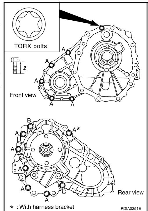
10. Separate front case and rear case. Then, remove front case by levering it up with a tire lever or the like.
