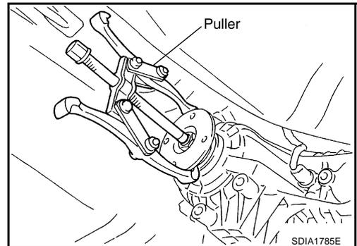
5. Remove the rear oil seal using a puller.
