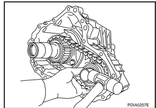
14. Install mainshaft bearing to front case, using a drift.
