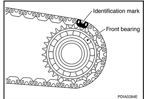
13. Install drive chain to mainshaft, and then install tap front drive shaft with plastic hammer. Press-fit rear bearing of front drive shaft to rear case.
