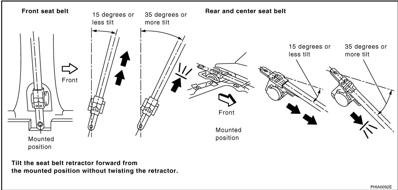
**15 degrees or less tilt** : Belt can be pulled out.
