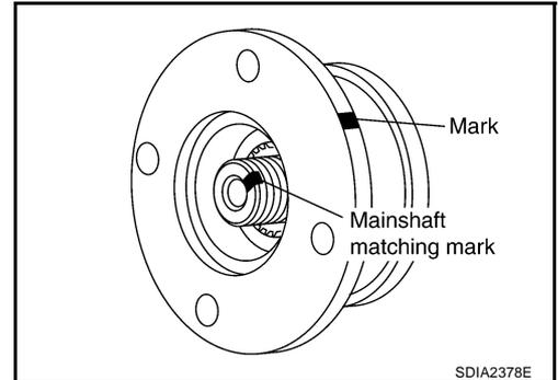
3. Using flange wrench, install the self-lock nut of companion flange and tighten to the specified torque. Refer to [TF-51, "COMPONENTS"](#).
