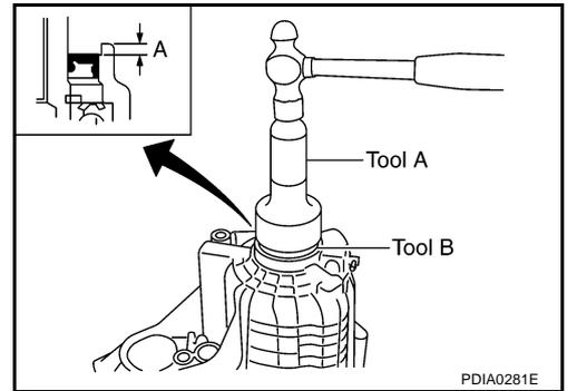
21. Install companion flange while align the matching mark of mainshaft with the mark of companion flange.
