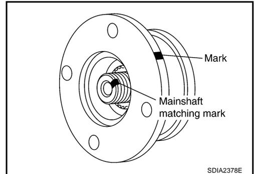
22. Tighten self-lock nut to the specified torque, with flange wrench. Refer to [TF-51, "COMPONENTS"](#).
