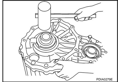
18. Tighten front case and rear case fixing bolts to the specified torque. Refer to [TF-51, "COMPONENTS"](#).
