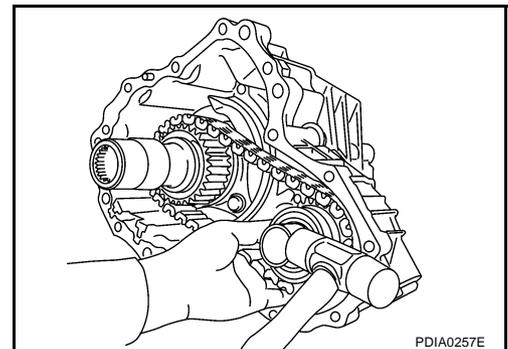
14. Remove oil gutter from rear case.
