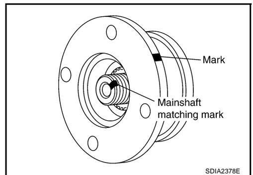
6. Remove companion flange, using a puller.
