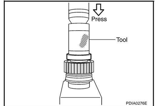
2. Install front drive shaft rear bearing, using a drift.
