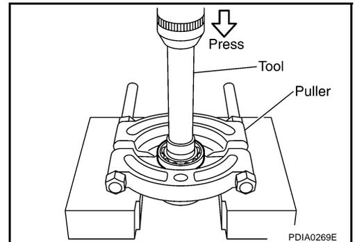
4. Remove front drive shaft rear bearing, using drift and puller.
