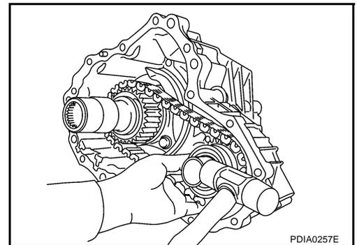
3. Remove front drive shaft front bearing, using drift and puller.
