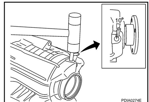
3. Install rear bearing to rear case, using a drift.
