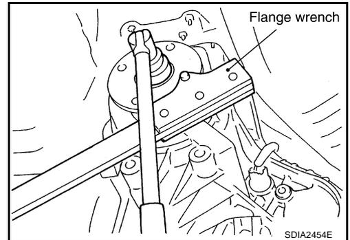
3. Put matching mark on the end of the mainshaft. The mark should be in line with the mark on the companion flange.
