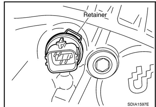
9. Set temperature sensor and tighten bolt to the specified torque. Refer to [TF-51, "COMPONENTS"](#).
