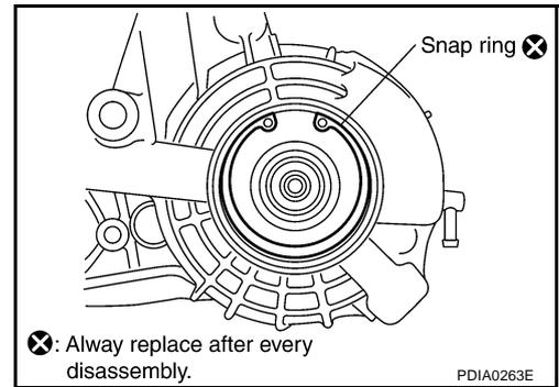
5. Install mainshaft assembly to rear case, using a drift.
