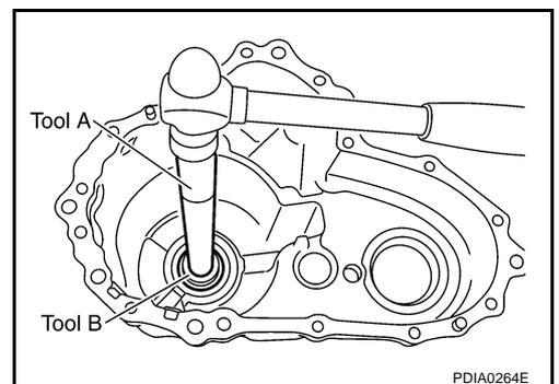
22. Remove baffle plate from rear case.
