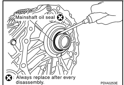
3. Remove front oil seal from front case, using a flat-bladed screwdriver.
