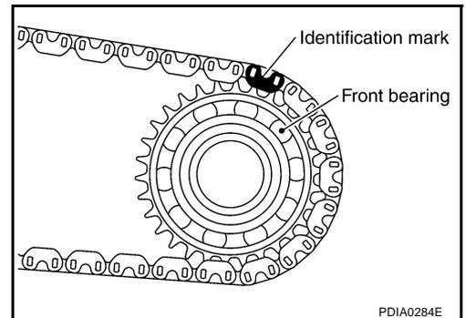
4. Install drive chain to mainshaft, and then install tap front drive shaft with plastic hammer. Press-fit rear bearing of front drive shaft to rear case.
