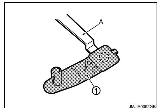
5. Remove foot grille. Refer to [VTL-13, "FOOT GRILLE : Removal and Installation"](#).
