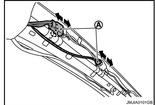
3. Remove front roof finisher mounting metal clips and pawls with a remover tool (A), and then remove front roof finisher (1).
