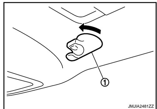
6. Remove mounting plastic clips (A) using a screwdriver (B) of front and rear assistance grips (1), and then remove assist grips.
