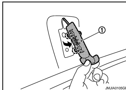
5. Remove trunk lid finisher mounting clips, and then remove trunk lid finisher inner.
