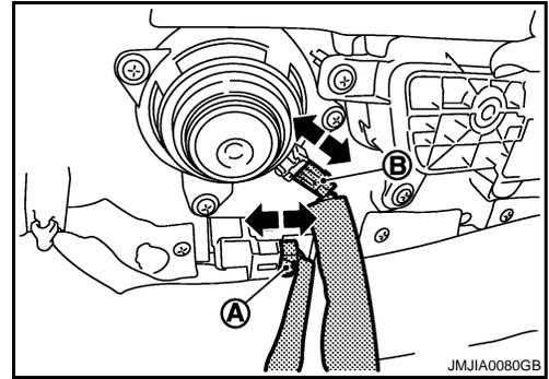
9. Disconnect the inside handle cable from door inside handle assembly. Refer to [DLK-231, "INSIDE HANDLE : Exploded View"](#).
