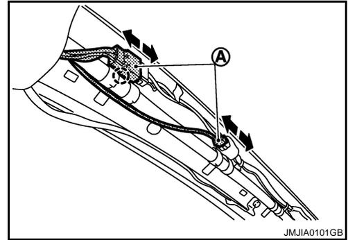
3. Remove front roof finisher mounting metal clips and pawls with a remover tool (A), and then remove front roof finisher (1).
