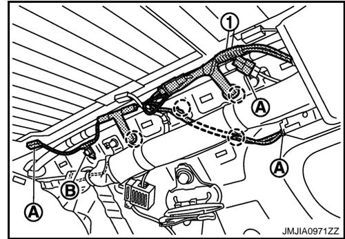
10. With a remover tool, remove body side mounting plastic clip from rear end of headlining.
