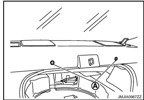
6. Remove rear seat striker cover fixing pawls, and then remove rear seat striker cover.
