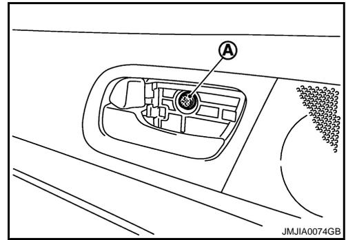
4. Remove armrest cap (1) with remover tool (A).
