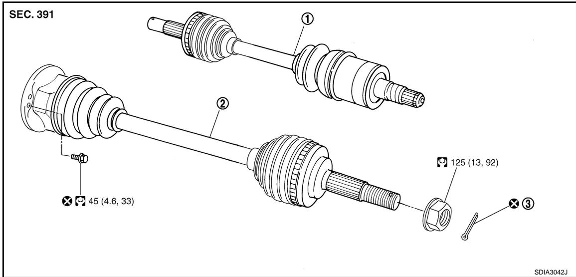
1. Drive shaft (right side)                      2. Drive shaft (left side)                      3. Cotter pin
