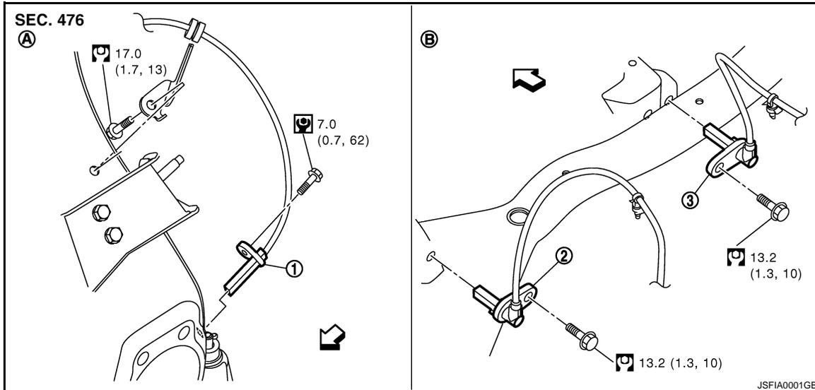
1. Front LH wheel sensor      2. Rear LH wheel sensor      3. Rear RH wheel sensor
