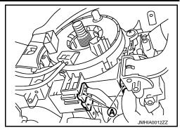
Remove the steering angle sensor. Refer to <u>BRC-117, "Removal and Installation"</u>.
