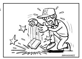
Replace the crash zone sensor of deployed the driver air bag and deployed the passenger air bag.
