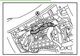
3. Remove the passenger air bag module mounting bolt and screws.
