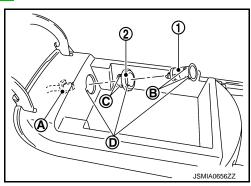
INSTALLATION Install in the reverse order of removal. **NOTE:** Align the cut outs of inner socket, ring, and center console assembly. INFOID:000000009163474
