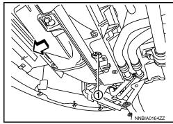
When draining all of engine coolant in the system, open water drain plugs on cylinder block. Refer to EM-58, "Setting (GT-R certified NISSAN dealer)".
