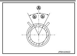
• To install hose clamps (1), check that the dimension (A) from the end of the paint mark (2) on the radiator hose to the hose clamp is within the reference value.
