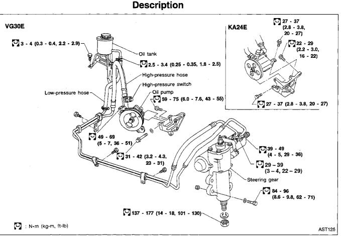
This power steering adopts spool valve control which was developed in a technical tie-up with the ZF Company.
