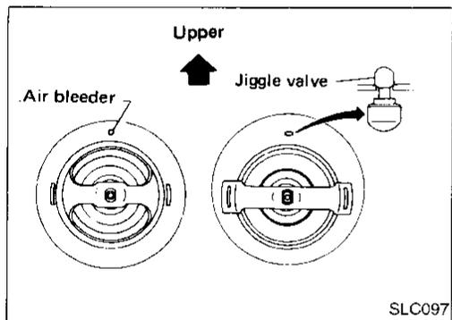
3. Install thermostat with jiggle valve or air bleeder at upper side.
