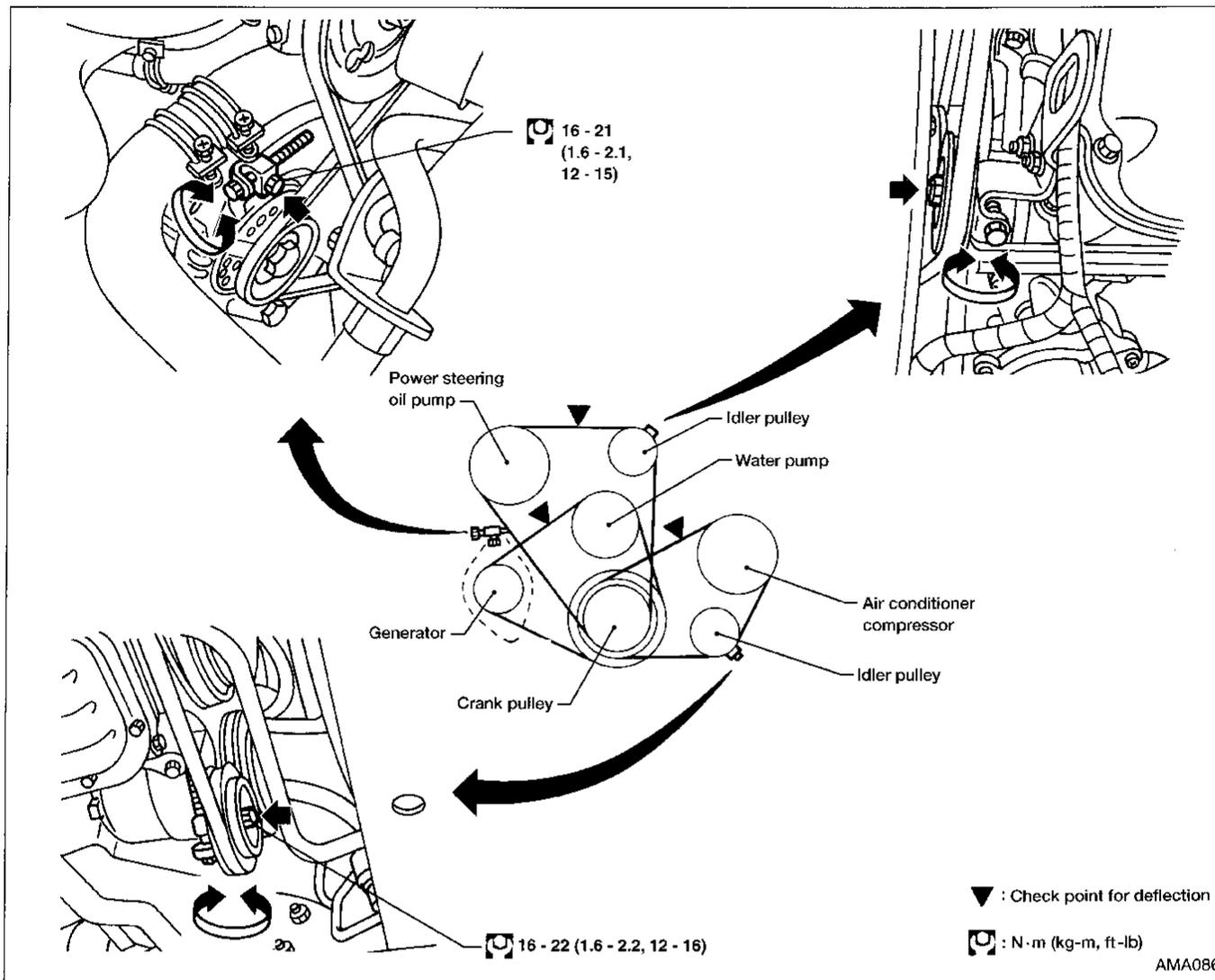
1. Inspect for cracks, fraying, wear and oil. If necessary, replace with a new one.
