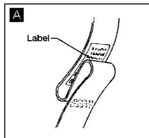
For front seat belt, shock absorber type belt has been used. Replace the belt when loop has been pulled out and "REPLACE BELT" is visible because this seat belt has a loop of webbing under the sleeve.
