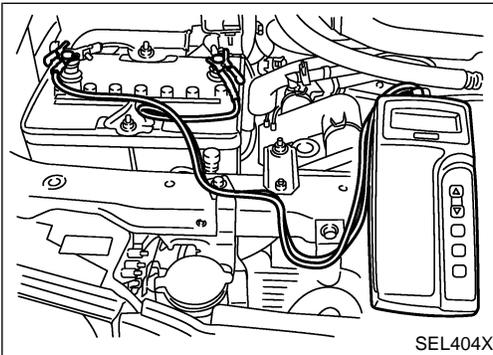
1. Turn off all loads on the vehicle electrical system. Clean or repair as necessary.
