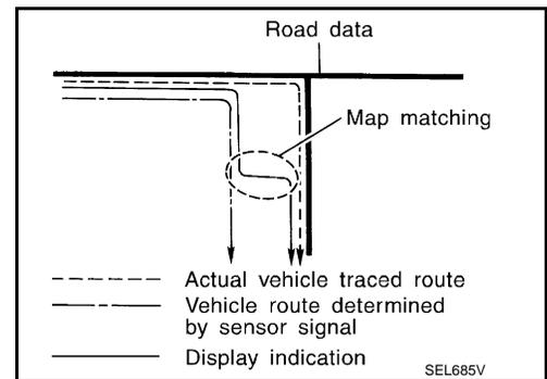
The vehicle position may not be corrected under the following circumstances and after driving for a certain time when GPS information is difficult to receive. In this case, the vehicle mark on the display must be corrected manually.
