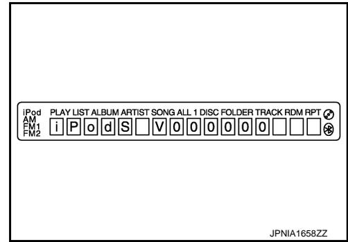
12. Press the "DISP TEXT" switch again to display the "iPodH" (iPod hardware version). "FFFFFF" is displayed when communication signals between the audio unit and iPod adapter include a malfunction.
